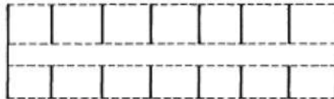
2.a cross-walls without longitudinal walls: unstable
