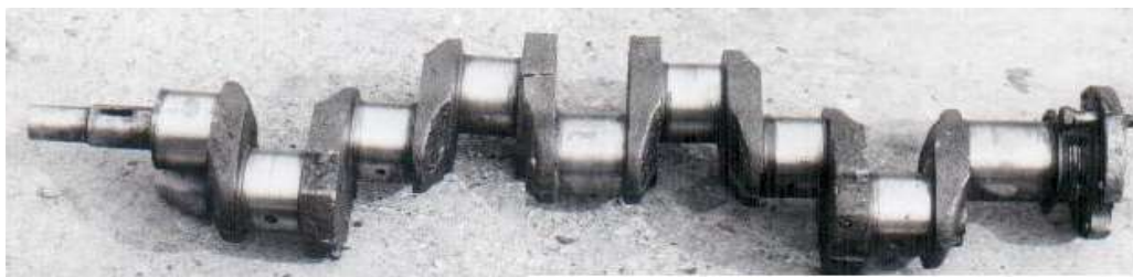
Fig. 1 Crankshaft of tractor 75 HP
