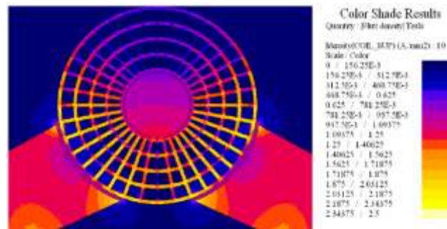
FIG 11: Magnetic scalar field shown by a color shade presentation. The results were calculated by applying the finite element method. The colors show different inductions \mu_0 H . The lower half cylinder shows high field intensities and the higher half low field intensities,
