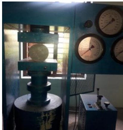
Fig.2.4 Compression testing machine for testing cylinder
