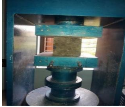
Fig 2.2 Compression testing machine for testing Cube
