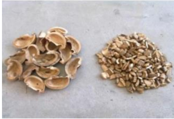
Fig 1 . Rubber seed shell (left side) and crushed rubber seed shell (right side)
