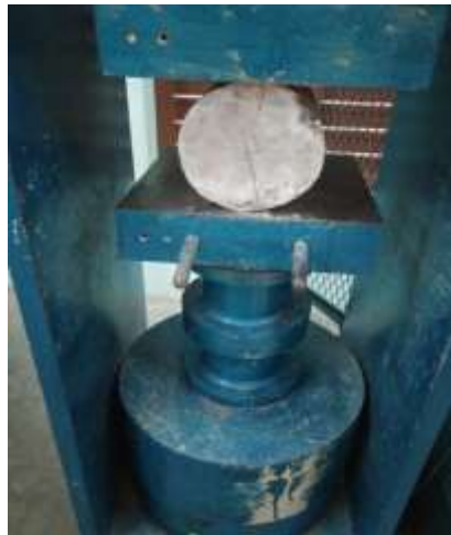
Fig 3 Split tensile strength test
