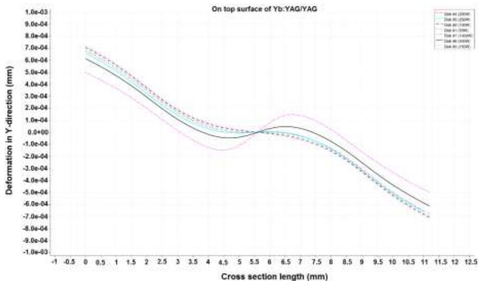
Figure 14. 2-dimensional comparison of Y-component of deformation inside the crystal for different pump powers.
