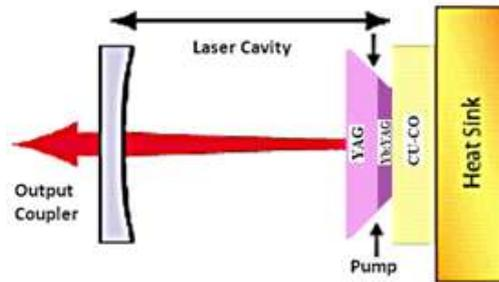
Figure 3. Schematic view of our disk configuration placed inside the linear cavity and cooling from the bottom surface.
