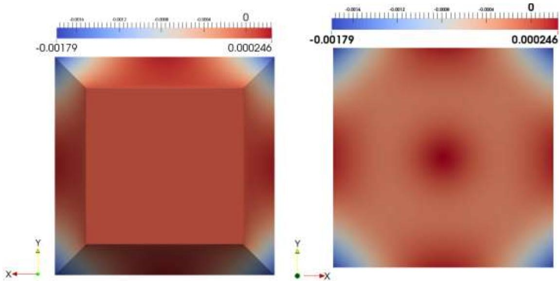
Figure 12. 3D deformation component distribution inside the crystal in Z-direction (parallel to the laser beam direction) from the cross section view on top and bottom surface of the crystal.
