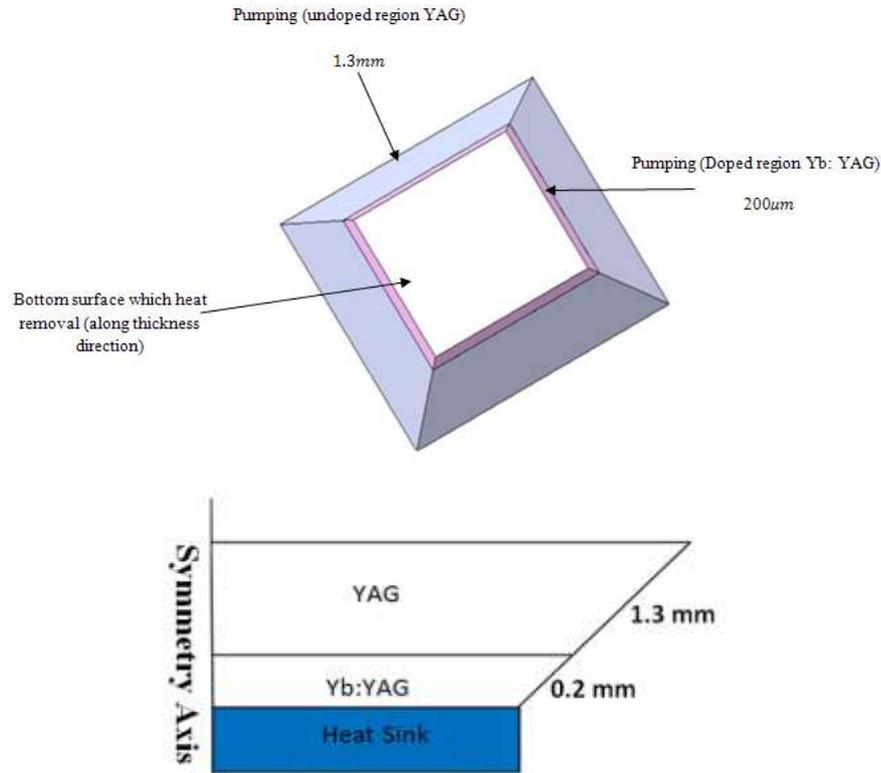
Figure 1. Isometric layout of the gain medium and half side cross-section view of the gain medium.
