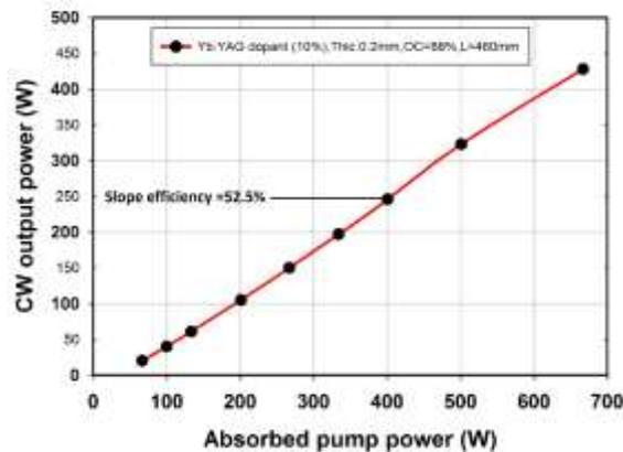
Figure 18. Absorbed pump power versus output power (slope efficiency) for Yb:YAG dopant of 10%
