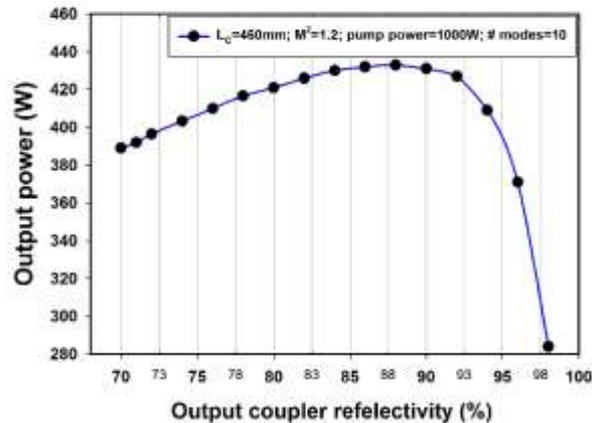
Figure 19. Optimizing the output coupler reectivity respect to the output power
