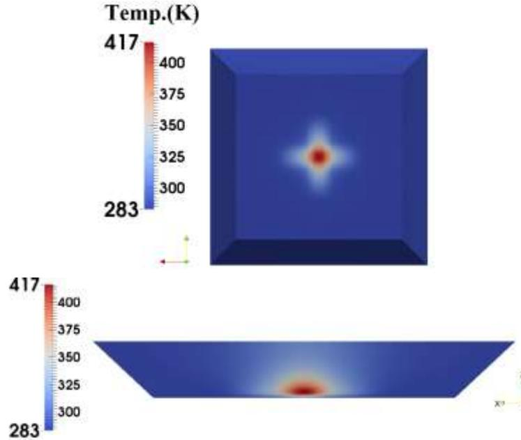
Figure 8. Temperature distribution profile inside the crystal from the bottom cross section view and from the side cross section view
