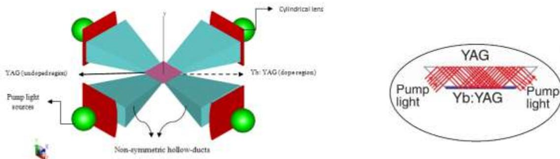
Figure 2. Isometric Schematic view of sources and four hollow ducts used for pumping the active medium from four slanted sides.
