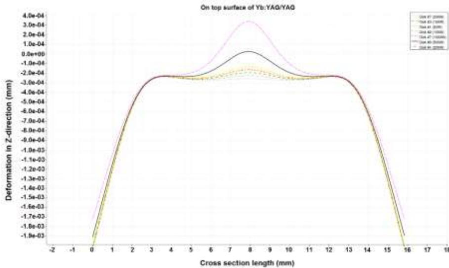
Figure 13. 2-dimensional comparison of Z-component deformation inside the crystal for different pump powers.
