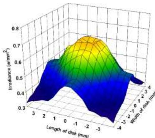
Figure 5. Pump light distribution profile inside the crystal obtained by ray tracing in TracePro.
