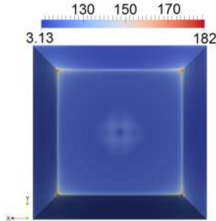
Figure 9. 3-dimensional Von Mises stress distributions on the bottom surface of the crystal.
