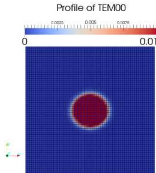
Figure 20. TEM00 profile on the front mirror
