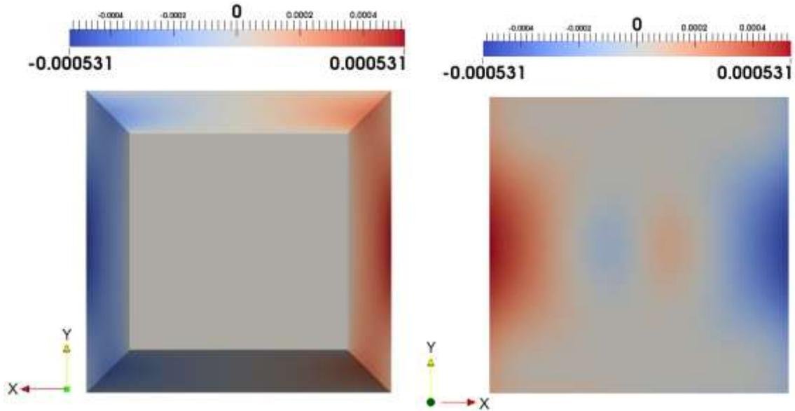
Figure 11. 3-dimensional deformation component distribution inside the crystal in X-direction (perpendicular to the laser beam direction) from the cross section view on top and bottom surface of the crystal.
