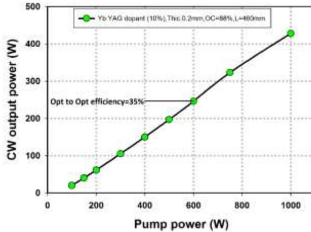
Figure 17. Pump power versus output power (optical to optical efficiency) for Yb:YAG dopant of 10%
