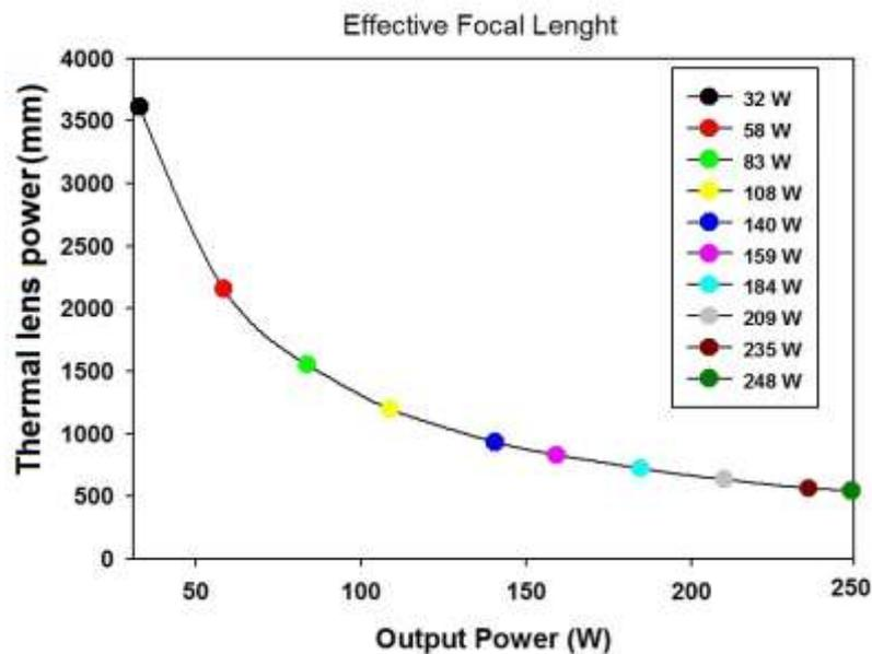
Figure 15. The effective focal length of the thermal lens corresponding to different output powers.
