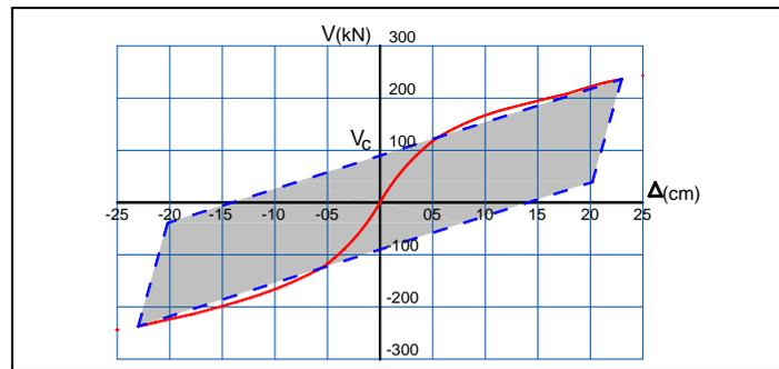
Figure 5. Hysteresis loop at maximum displacement..
