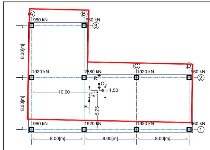
Figure 4. Building displacement in plan.
