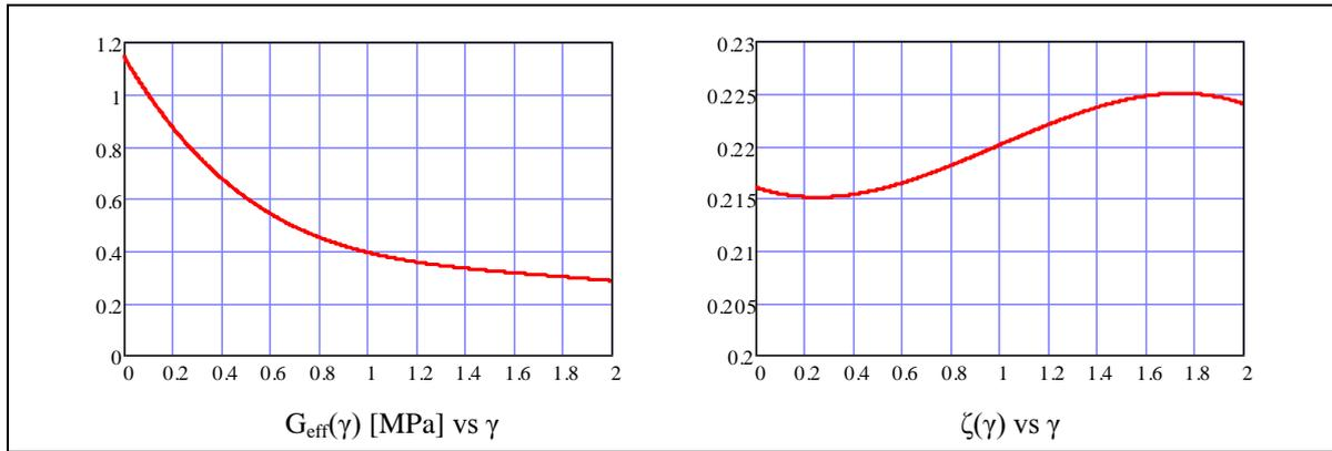
Figure 1. Elastomeric characteristics for high dumping rubber with normal hardness
