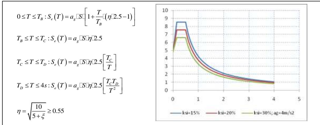
Figure 3. Elastic acceleration spektra according Eurocode-8
