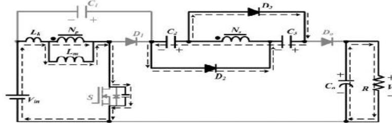
Figure.4. Current flowing path of proposed converter CCM Mode III operation.
