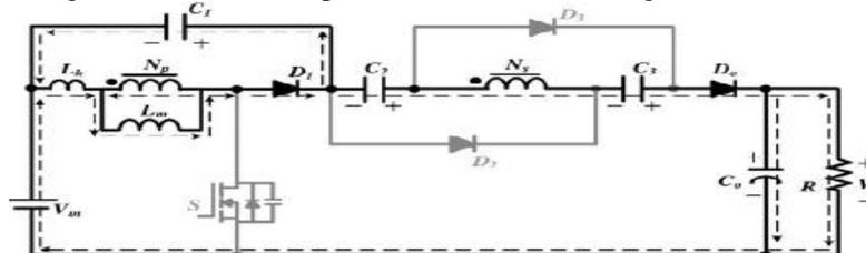
Figure.6. Current flowing path of proposed converter CCM Mode V operation
