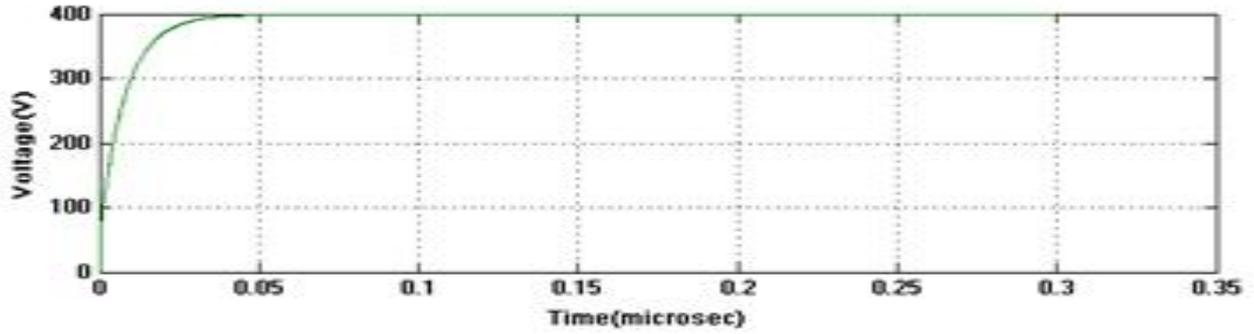
Figure.14. Output voltage waveform for proposed converter in CCM operation
