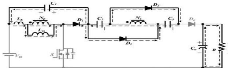
Figure.5. Current flowing path of proposed converter CCM Mode IV operation
