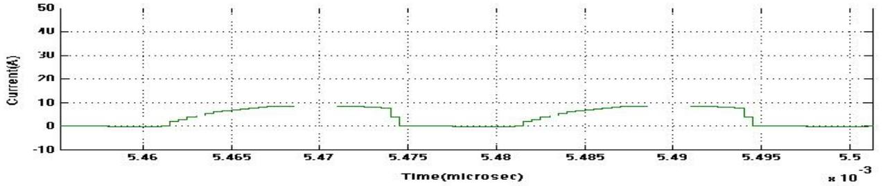
Figure.20 Output current waveform for proposed converter in CCM operation at  $I_{d3}$ .
