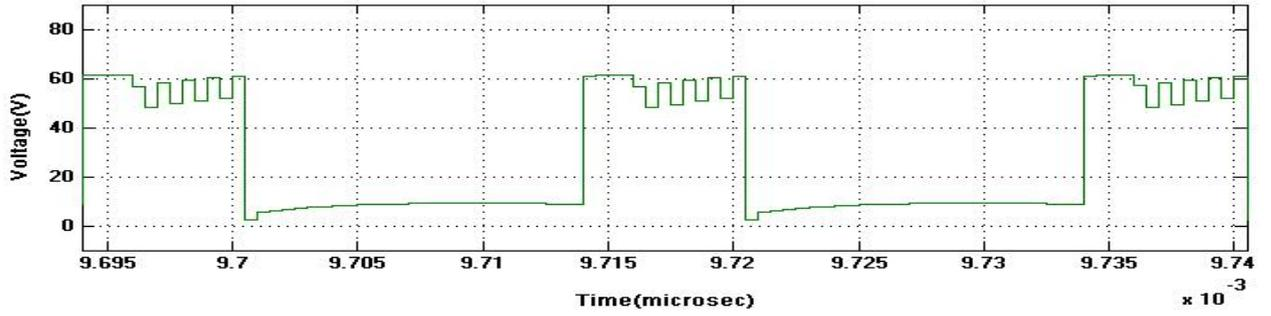
Figure.18. Output voltage waveform for proposed converter in CCM operation at  $V_{ds}$ .
