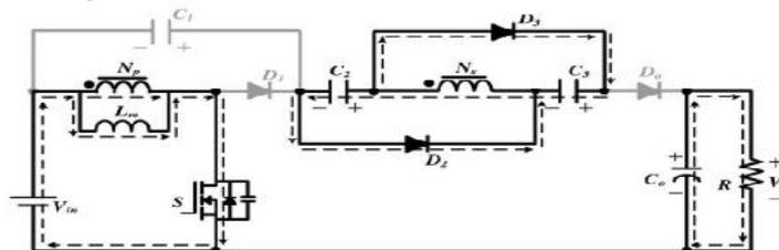
Figure.9. Current flowing path of proposed converter DCM Mode I operation
