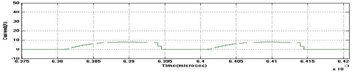
Figure.19 Output current waveform for proposed converter in CCM operation at  $I_{d2}$ .
