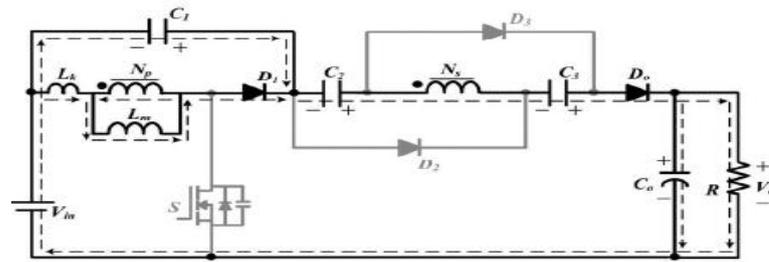
Figure.7. Current flowing path of proposed converter CCM Mode VI operation
