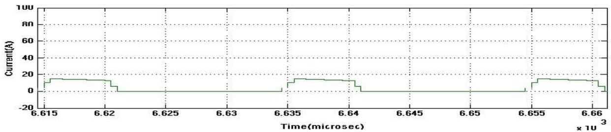
Figure.22. Output current waveform for proposed converter in CCM operation at  $I_{d0}$ .
