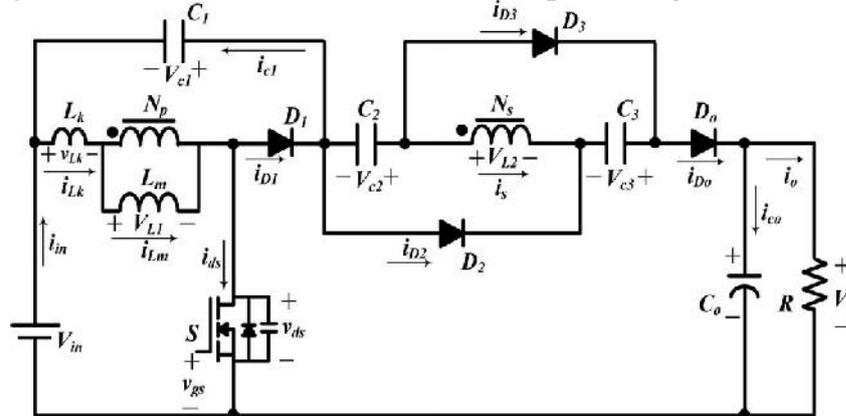
Figure.1. Circuit Configuration of the proposed converter
