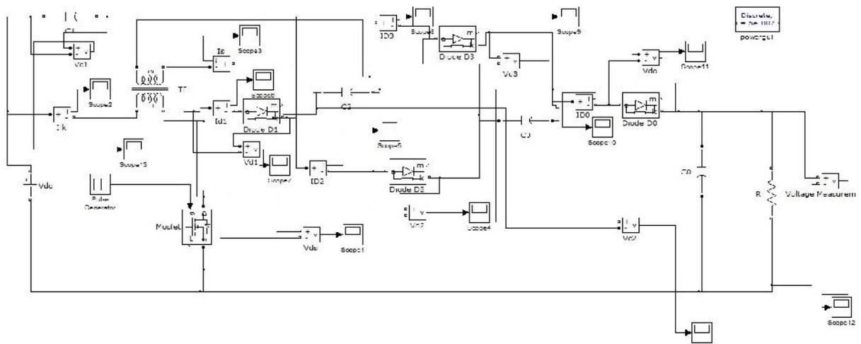
Figure.13 MATLAB/Simulink Model of the Proposed Converter under Full-Load condition  $P_o=400W$ .
