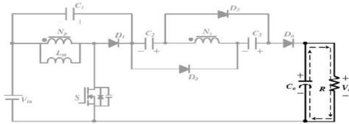
Figure.11. Current flowing path of proposed converter DCM Mode III operation
