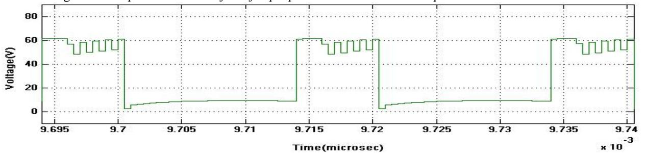
Figure.21. Output voltage waveform for proposed converter in CCM operation at  $V_{ds}$ .
