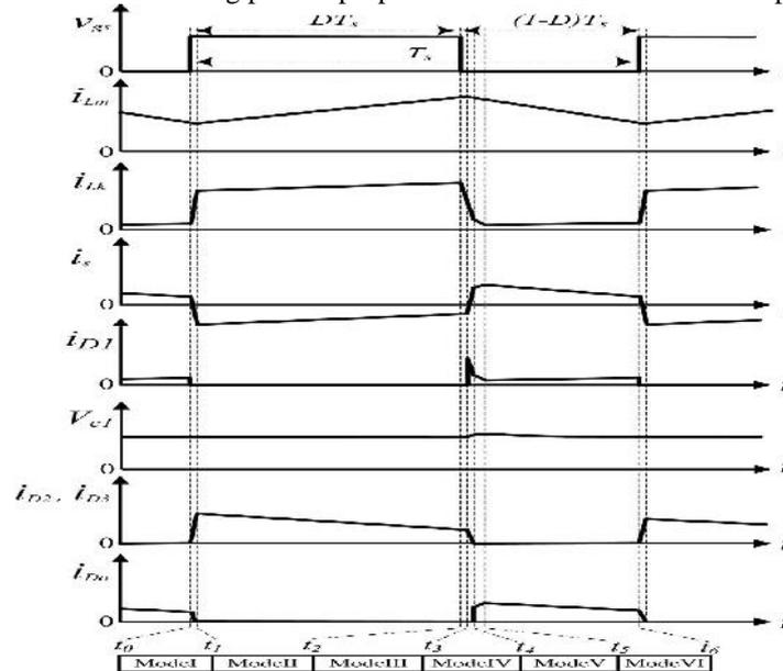
Figure.8. Some typical key waveforms of the proposed converter at CCM operation.
