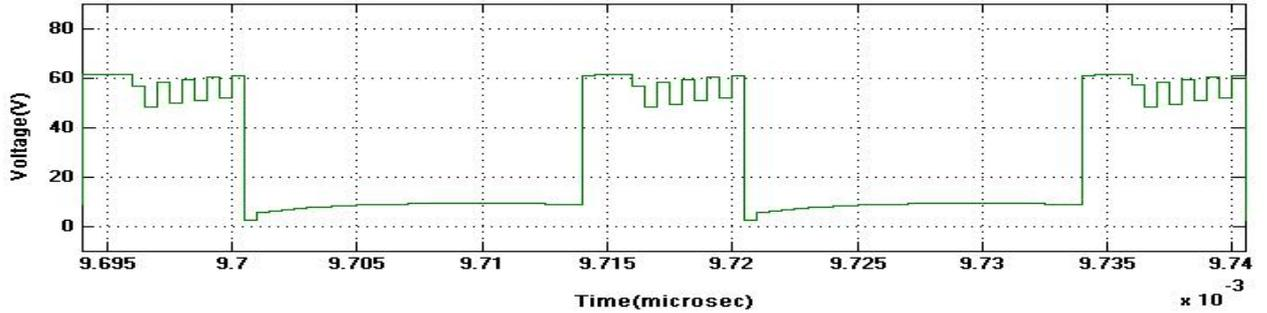
Figure.15. Output voltage waveform for proposed converter in CCM operation at  $V_{ds}$ .
