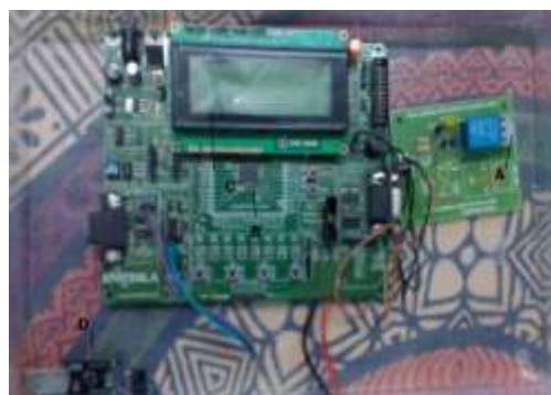
Fig :- Receiver section(A. Motor connections, B. Arm processor, C. Display , D. RF module)
