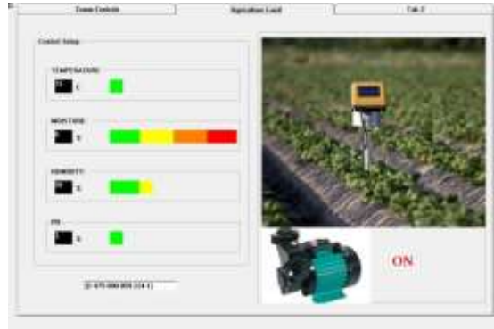
Fig 10 :- The values of sensors below the threshold values motor is START or ON
