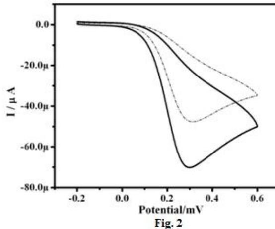
**Figure. 2** Cyclic voltammogram of 0.1 mM AA at solid line for modified carbon paste electrode prepared with Montmorillonite K<sub>10</sub>-clay (MMCPE) and at dotted line for bare CPE.
