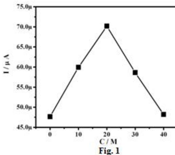
**Figure. 1** Effect of concentration of Montmorillonite K<sub>10</sub>-clay on anodic peak current ( $I_{pa}$ ) in 0.1 mM AA and 0.1 M phosphate buffer solution Scan Rate: 50 mVs<sup>-1</sup>
