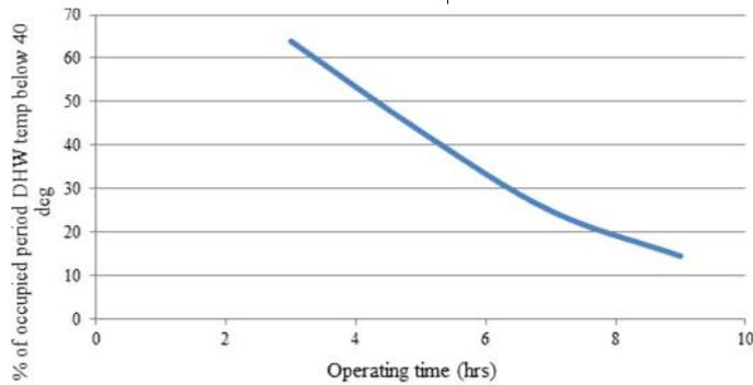
Fig 5 Effect of reducing pump running time (start time at 7am) on proportion of occupied period DHW temp < 40 deg
