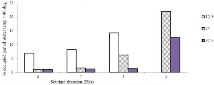
Fig 19 Effect of reducing set time duration & % of PCM with 5am as start time on % occupied period water temp < 40 deg (PCM in water tank)
