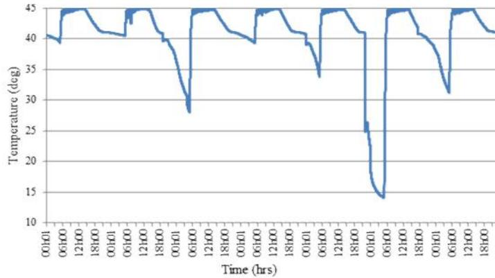
Fig 10 DHW tank water temp profile over simulation period (5.00 - 14.00, 12.5% PCM)
