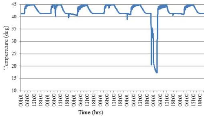
Fig 15 DHW tank water temp profile over simulation period (3.00 - 12.00, 37.5% PCM)
