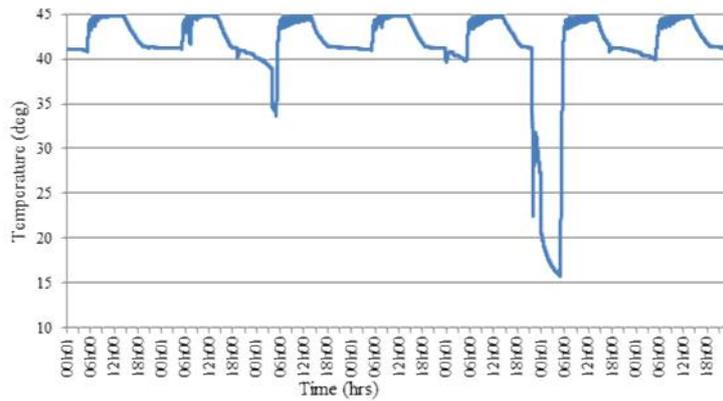
Fig 11 DHW tank water temp profile over simulation period (5.00 - 14.00, 25% PCM)
