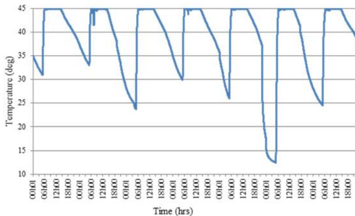
Fig. 6 DHW tank water temp profile over simulation period (5.00 - 14.00)
