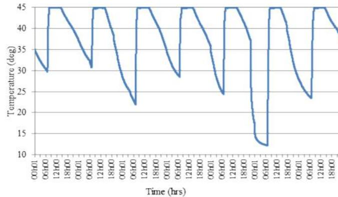
Fig. 2 DHW tank water temp profile over simulation period (7.00 - 14.00)
