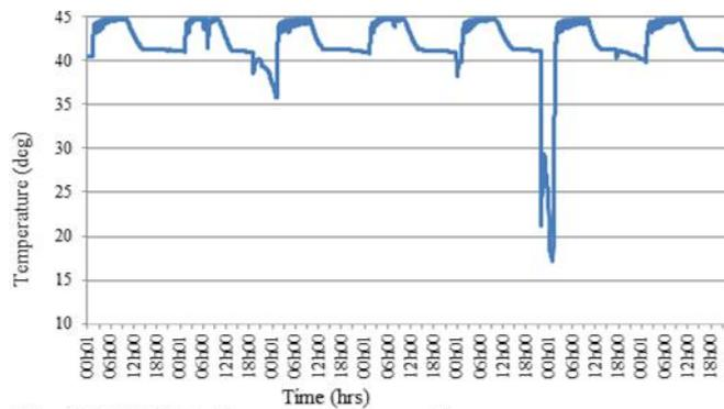
Fig 16 DHW tank water temp profile over simulation period (1.00 - 10.00, 25% PCM)
