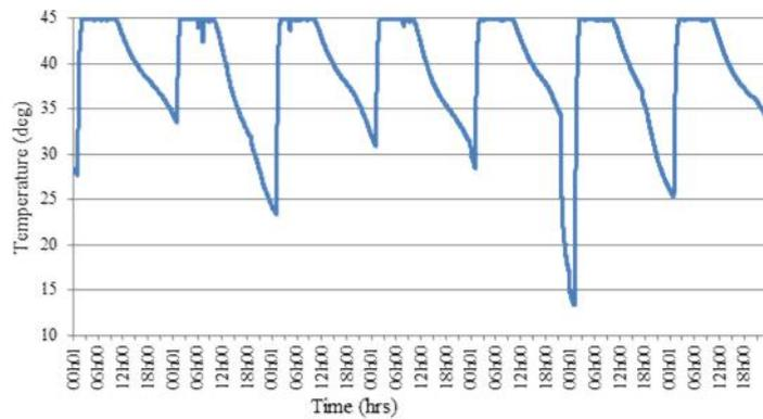
Fig 8 DHW tank water temp profile over simulation period (1.00 - 10.00)
