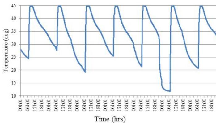
Fig 4 DHW tank water temp profile over simulation period (7 - 10)
