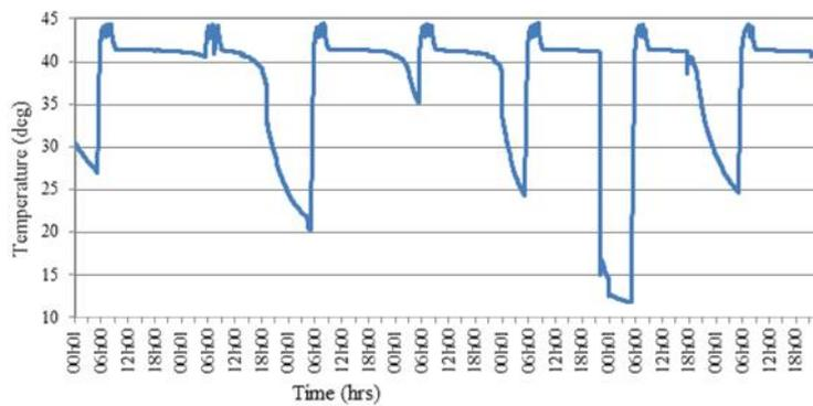
Fig 21 DHW tank water temp profile over simulation period (5.00 - 8.00, 37.5% PCM)
