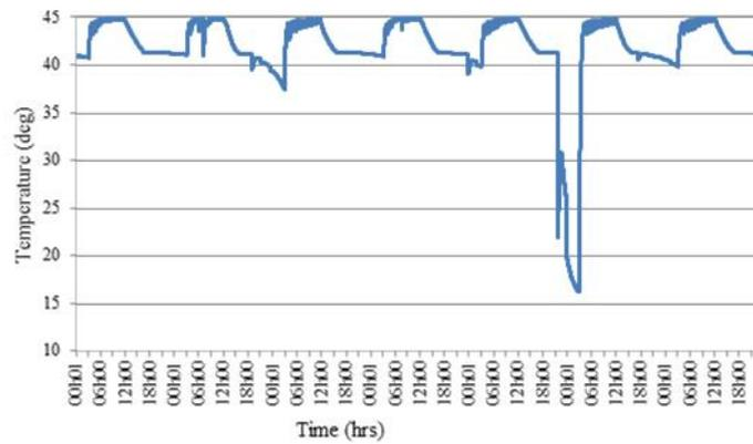
Fig 14 DHW tank water temp profile over simulation period (3.00 - 12.00, 25% PCM)
