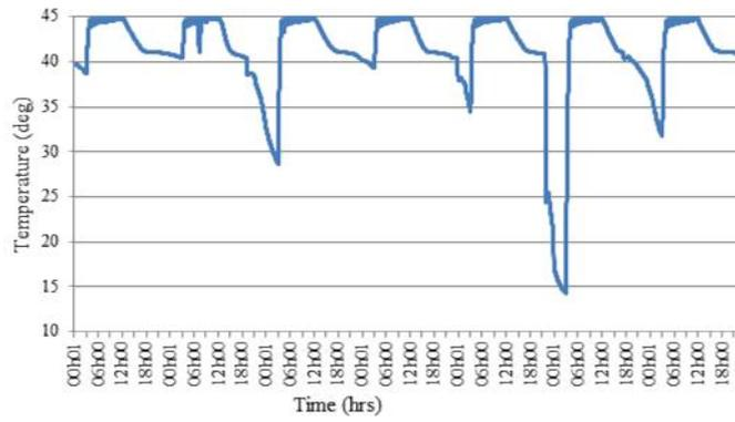
Fig. 13 DHW tank water temp profile over simulation period (3.00 - 12.00, 12.5% PCM)
