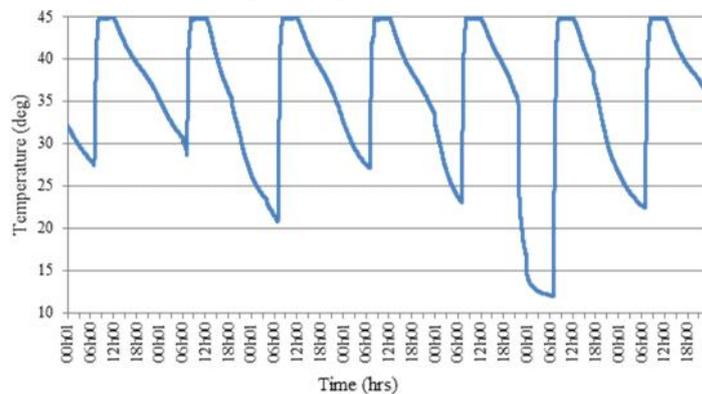
Fig 3 DHW tank water temp profile over simulation period (7.00 - 12.00)
