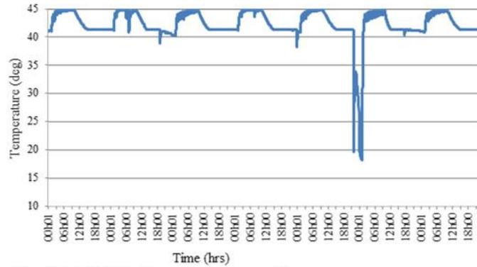
Fig 17 DHW tank water temp profile over simulation period (1.00 - 10.00, 37.5% PCM)
