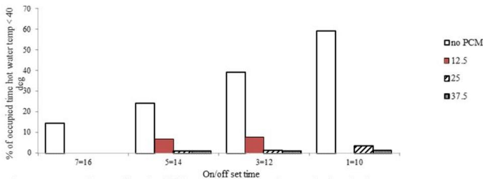
Fig 18 Comparison of back shifting effect on % of occupied period water temp < 40 deg for no-PCM and different percentage of PCM in DHW tank
