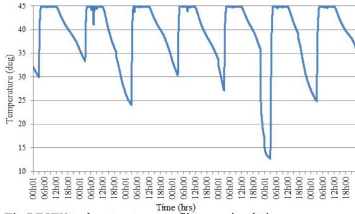
Fig 7 DHW tank water temp profile over simulation period (3.00 - 12.00)
