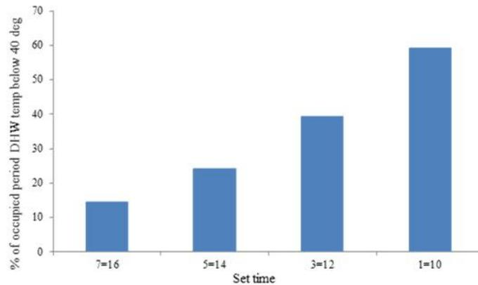
Fig 9 Effect of back shifting set time duration on % of occupied period DHW temp below 40 deg
