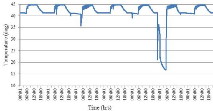
Fig 12 DHW tank water temp profile over simulation period (5.00 - 14.00, 37.5% PCM)
