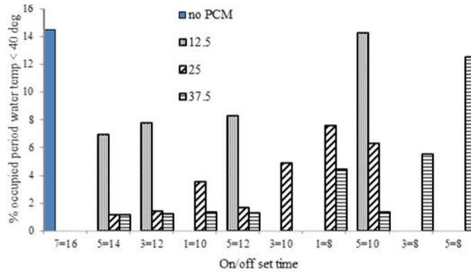
Fig 20 Comparison of Effect of on/off set time and % PCM on % occupied period wter temp < 40 deg
