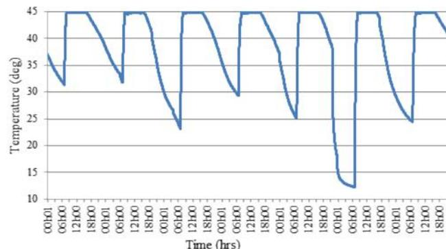
Fig.1 - DHW tank water temp profile over simulation period (7.00 - 16.00)
