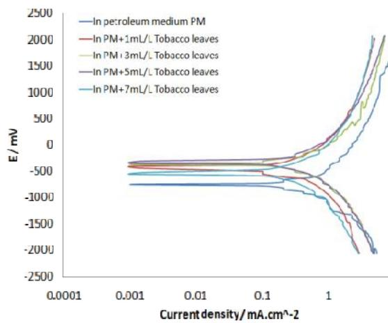
Figure 3. Tafel plots of carbon steel in petroleum medium in the presence of four concentrations of tobacco extract at 50°C.
