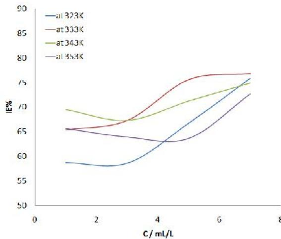
Figure 4. Relationship between inhibition efficiencies and concentrations of *Tobacco* extract at four temperatures.
