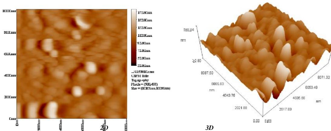
Figure 8. AFM images of the surface of steel immersed in petroleum medium (blank).
