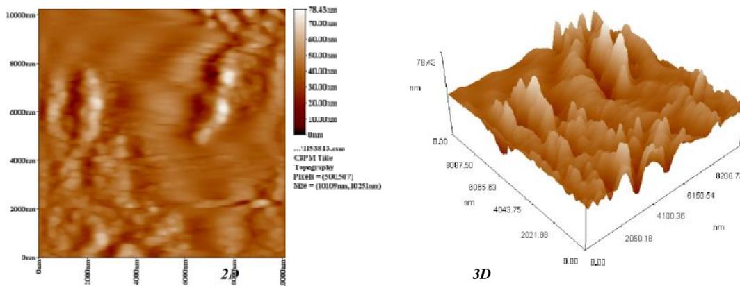
Fig. (9): AFM images of the surface of steel immersed in petroleum medium containing 7mL/L Tobacco extract.
