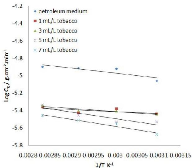
Figure 6. Arrhenius plots of the corrosion rate for steel in petroleum medium in absence and presence of Tobacco extract.
