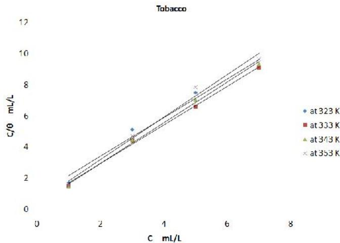
Figure 5. Langmuir adsorption plots for steel in petroleum medium with different concentrations of *Tobacco* extracts at four temperatures.
