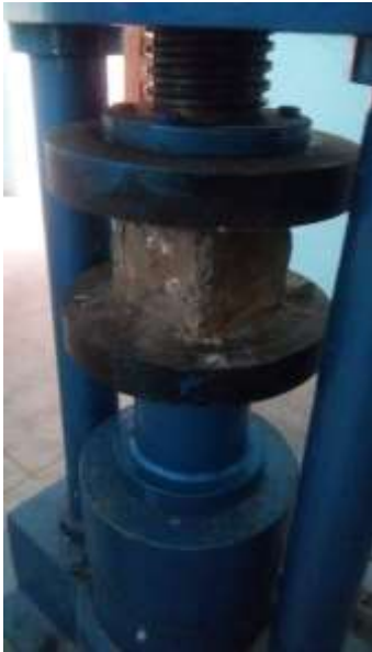
Figure 1 Compression Testing of cube specimen
