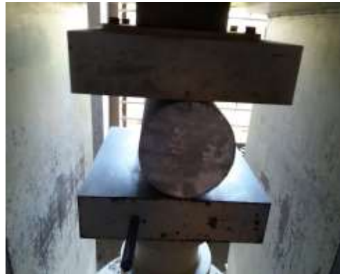
Figure 2 Split tensile test on cylinders
