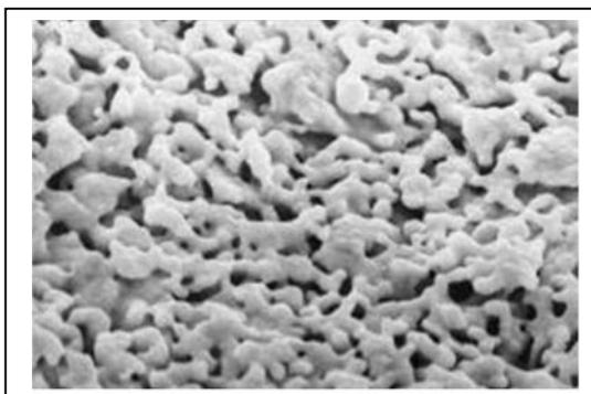
Figure 4. SEM micrograph of AgNp's synthesized by AL plant extract
