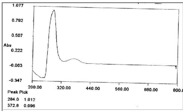
Fig 3 UV-Vis absorption spectrum of NPM3DMPO
