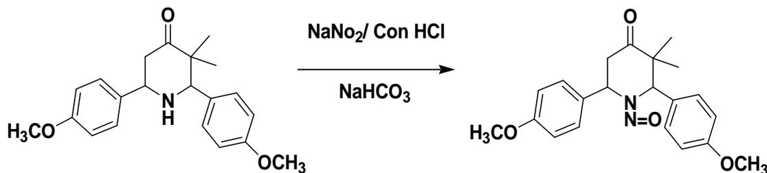
**Scheme – 1** The schematic representation for the preparation of NPM3DMPO
