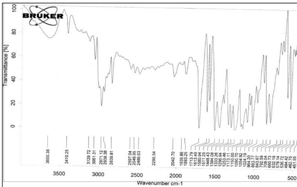
**Fig 4** FT-IR spectrum of NPM3DMPO
