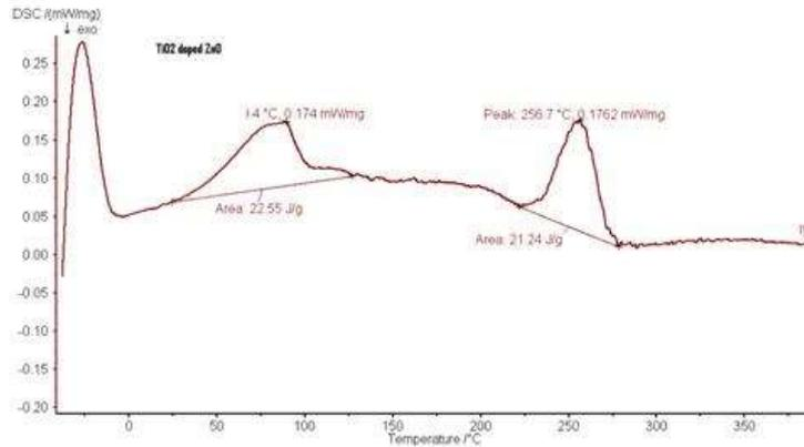
Figure 3. DSC curve of ZnO:TiO<sub>2</sub> Nanocomposite
