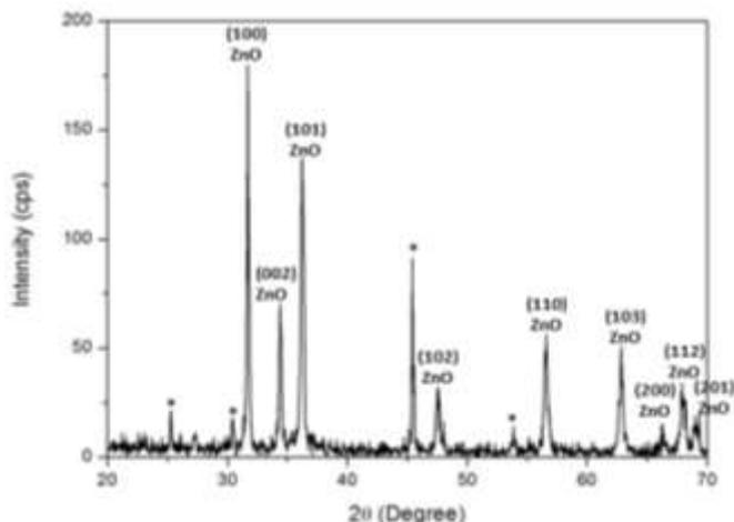
Figure 1. XRD pattern recorded from ZnO :TiO<sub>2</sub>nanocomposite
