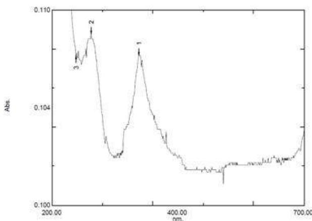
Figure 2. UV-Vis. Absorption spectrum of ZnO/ TiO<sub>2</sub> Nanocomposite
