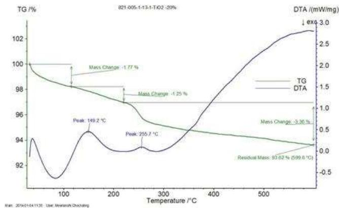
Figure 4. TG/DTA curves of ZnO: TiO<sub>2</sub>Nanocomposite
