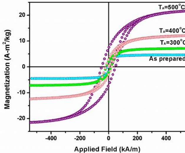
Figure 4. Magnetic behaviour of annealed Co<sub>50</sub>Ag<sub>50</sub> sample
