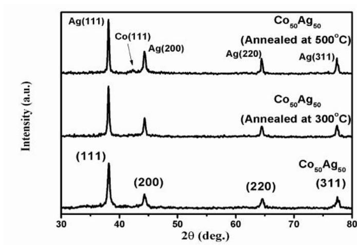
Figure 1. XRD patterns of  $\text{Co}_{50}\text{Ag}_{50}$  sample annealed at 300 °C and 500 °C
