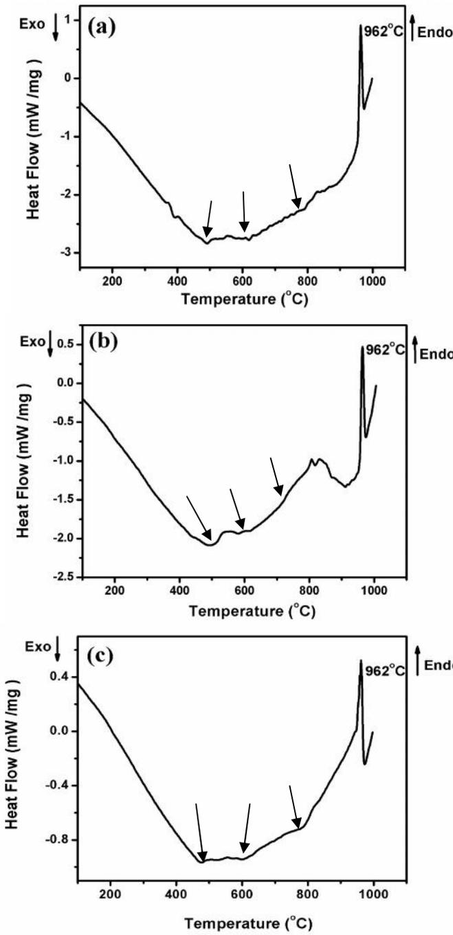
Figure 2. DSC plots of a)  $\text{Co}_{25}\text{Ag}_{75}$  b)  $\text{Co}_{50}\text{Ag}_{50}$  and c)  $\text{Co}_{75}\text{Ag}_{25}$  samples.
