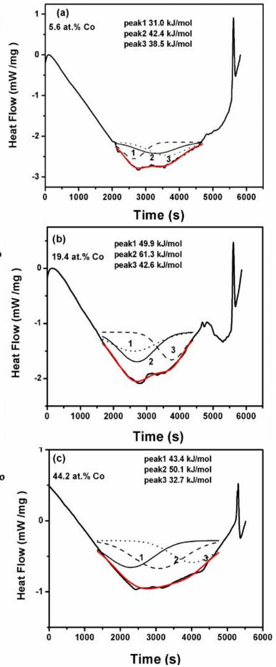
Figure 3. DSC traces resolved into 3 peaks representing the three processes
