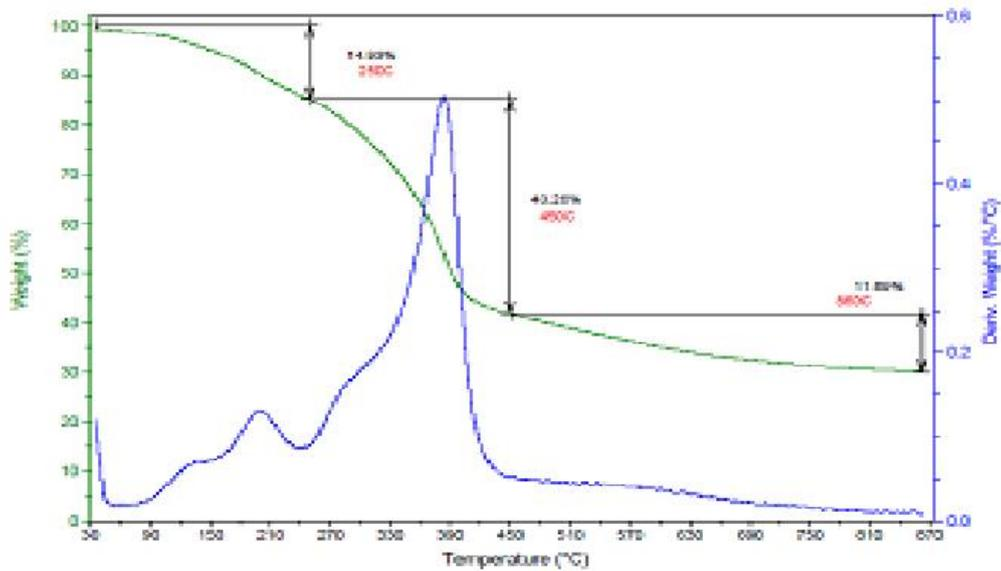
Figure.4 TGA of Polyester-ZnO nanoparticles
