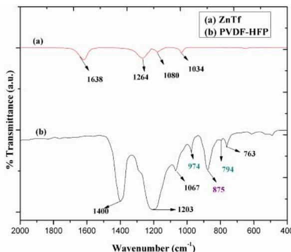
Fig. 4 FTIR spectra of of PVDF-HFP polymer and Zinc triflate salt in the spectral range 2000-400 cm<sup>-1</sup>
