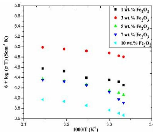
Figure 2. Temperature dependence of conductivity for various compositions of PVDF-HFP/(ZnTf)/Fe<sub>2</sub>O<sub>3</sub> CPEs at room temperature (300 K)
