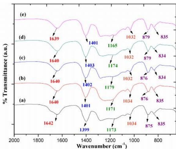
Fig. 3 FTIR spectra of various compositions of PVDF-HFP/(ZnTf)/Fe<sub>2</sub>O<sub>3</sub> CPEs in the spectral range 2000-800 cm<sup>-1</sup>
