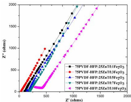
Figure 1. Typical complex impedance plots for various compositions of PVDF-HFP/(ZnTf)/Fe<sub>2</sub>O<sub>3</sub> CPEs at room temperature (300 K)
