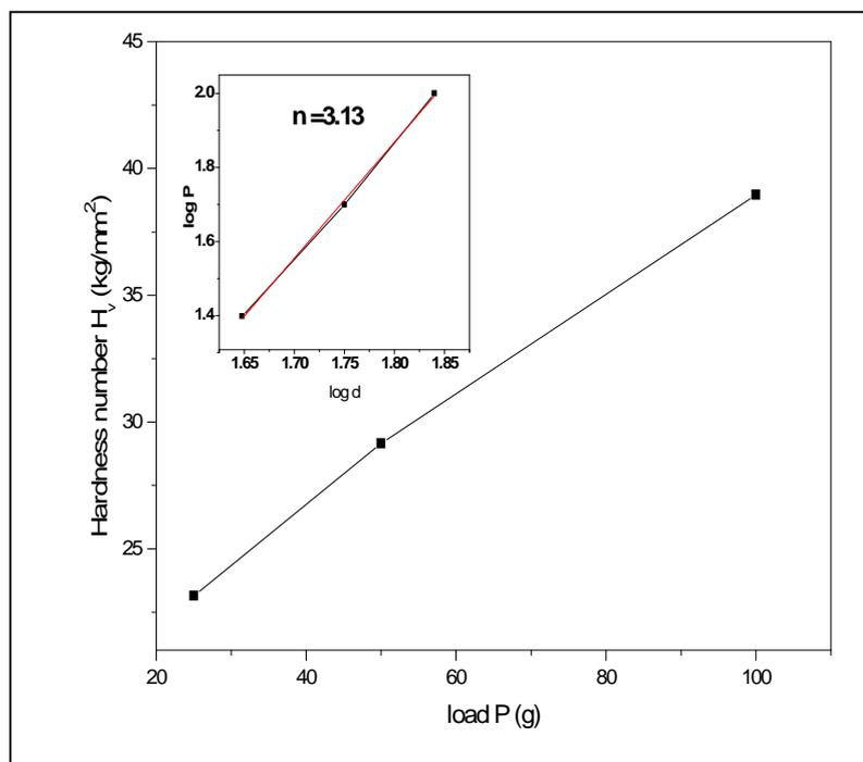
Figure 2. Variation of hardness number with load for beta-alanine crystal
