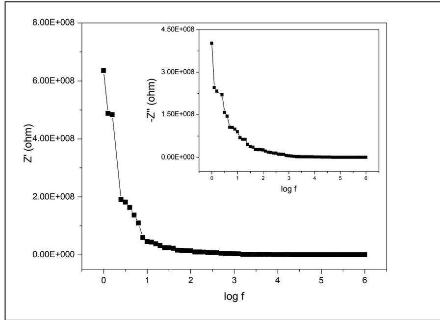
Figure 3. Variation of real part of impedance of the beta-alanine crystal with frequency.
