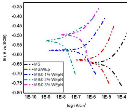
Figure 5 Potentiodynamic polarization curves of MS, WEp coated MS and WEpN composites coated MS
