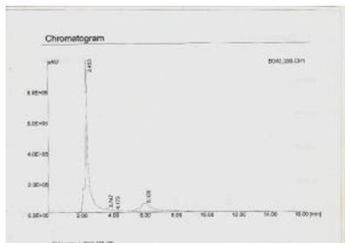
Fig 5: HPLC separation of siderophores isolated from an iron limited culture filtrate of *Penicillium chrysogenum*, Siderophores were separated on a C<sub>18</sub> reversed phase column and monitored at 220nm.
