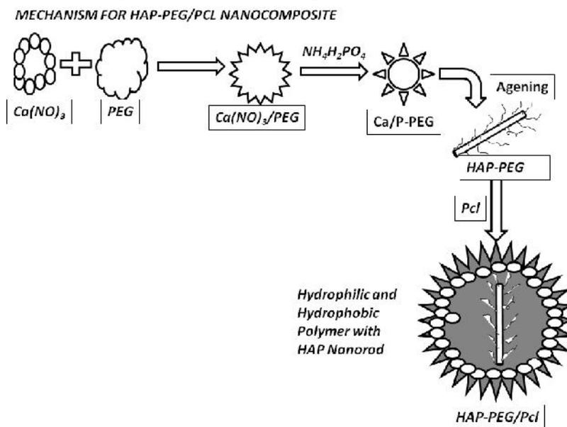
0.5g of PCL was dissolved in chloroform and HAP-PEG nanorods were added and then it was ultrasonicated for 15 min. In order to prepare HAP-PEG/PCL nano composites, the chloroformic solution was poured on to a petridish and dried under vacuum.
