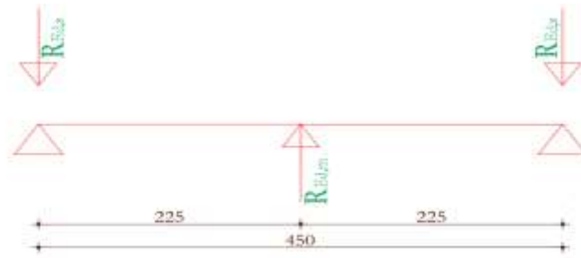
Figure 4. Scheme for main beam
