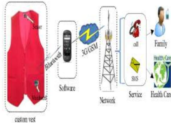
**Fig5: System architecture for fall detection**
