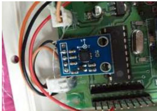
**Fig3: 3-axis accelerometer.**
